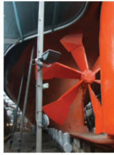
ABOVE The ss Great Britain was the first major steamship to take advantage of screw propulsion rather than the traditional paddles
